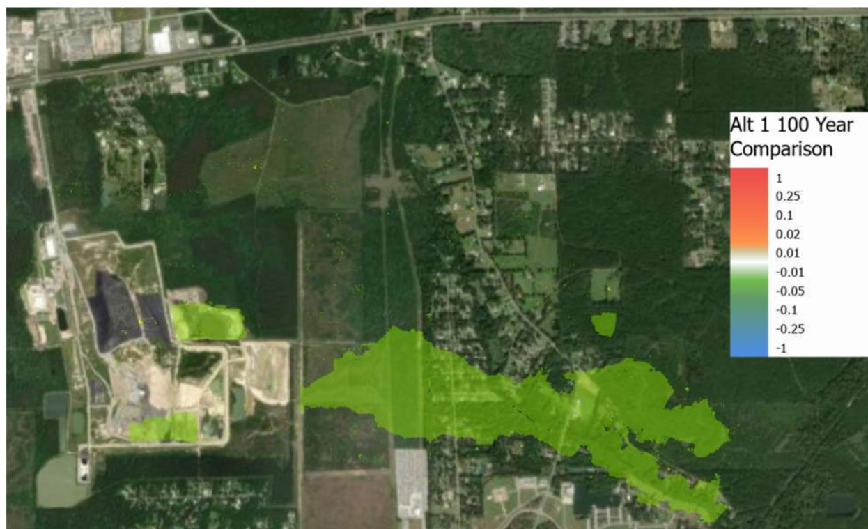
Figure 15c – Water Surface Elevation Difference (Existing vs. Proposed 1) for Southern Portion of Model
