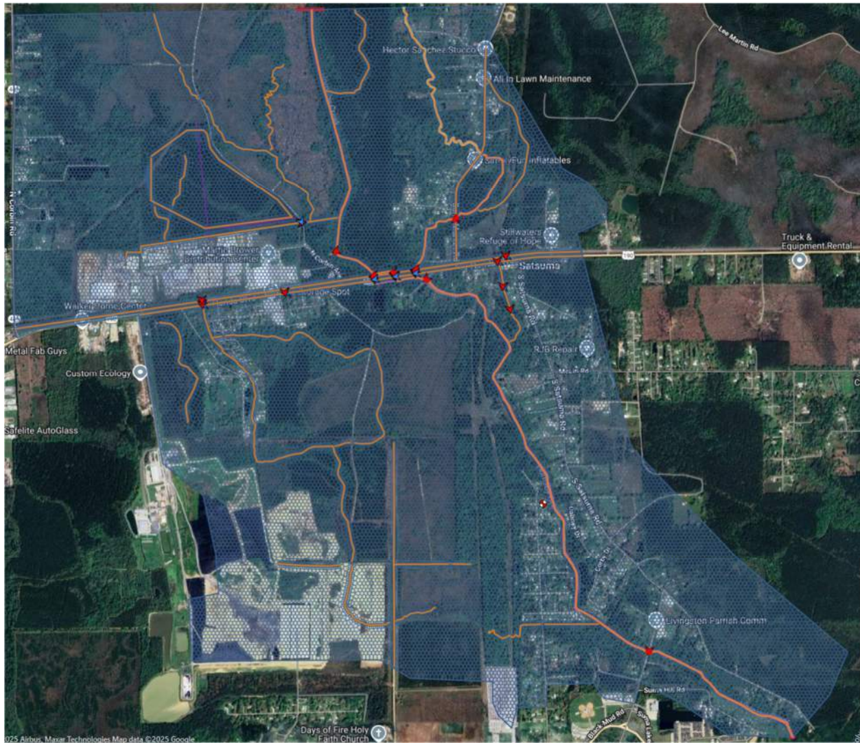
*Red and blue arrows represent culverts and SA-2D connections respectively Figure 2 – 2D Area of HEC-RAS Model
