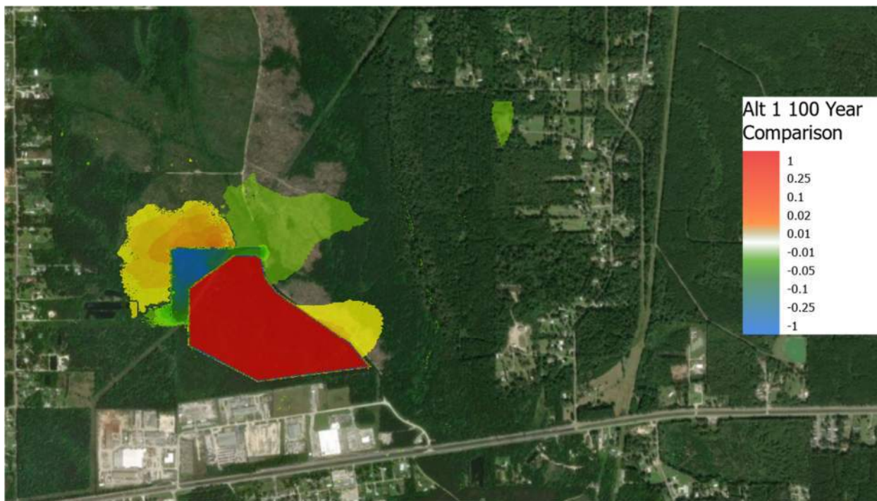
Figure 15a – Water Surface Elevation Difference (Existing vs. Proposed 1) for Northern Portion of Model
