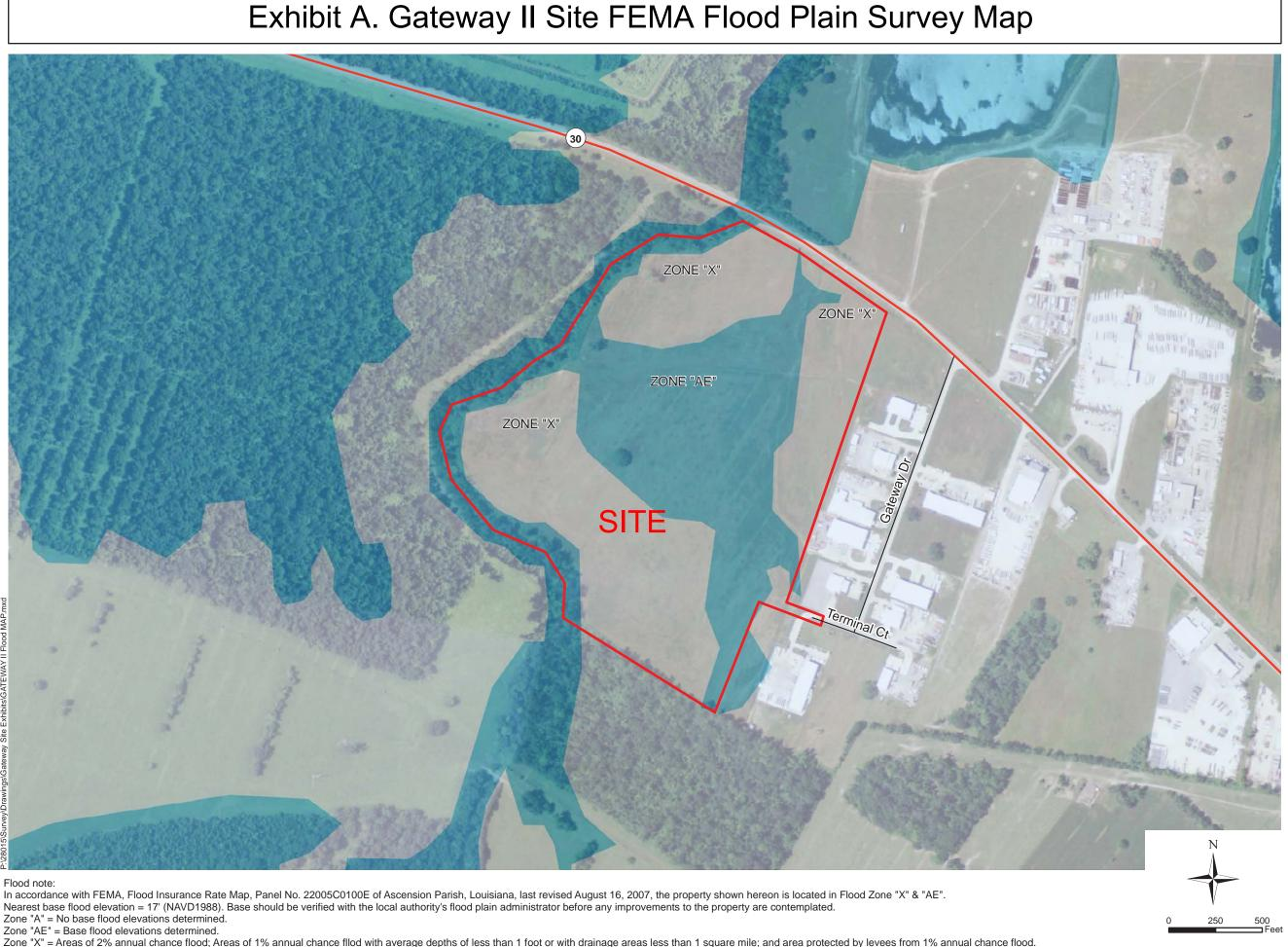
Nearest base flood elevation = 17' (NAVD1988). Base should be verified with the local authority's flood plain administrator before any improvements to the property are contemplated. Zone "A" = No base flood elevations determined.
