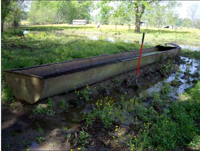
**Figure 32.** A split boiler shell on Angel Ranch property, 3.2 km southeast of Bouvard Sugar Mill site (16PC110), facing west. Note the rivets joining the various sections of the shell. The shell has been split in half horizontally, and end plates as well as lengths of small-diameter pipe (to cover the sharp edges) have been welded on. The sheet metal at the top of the far end has been added to protect the water intake. Photograph taken 15 April 2013.
