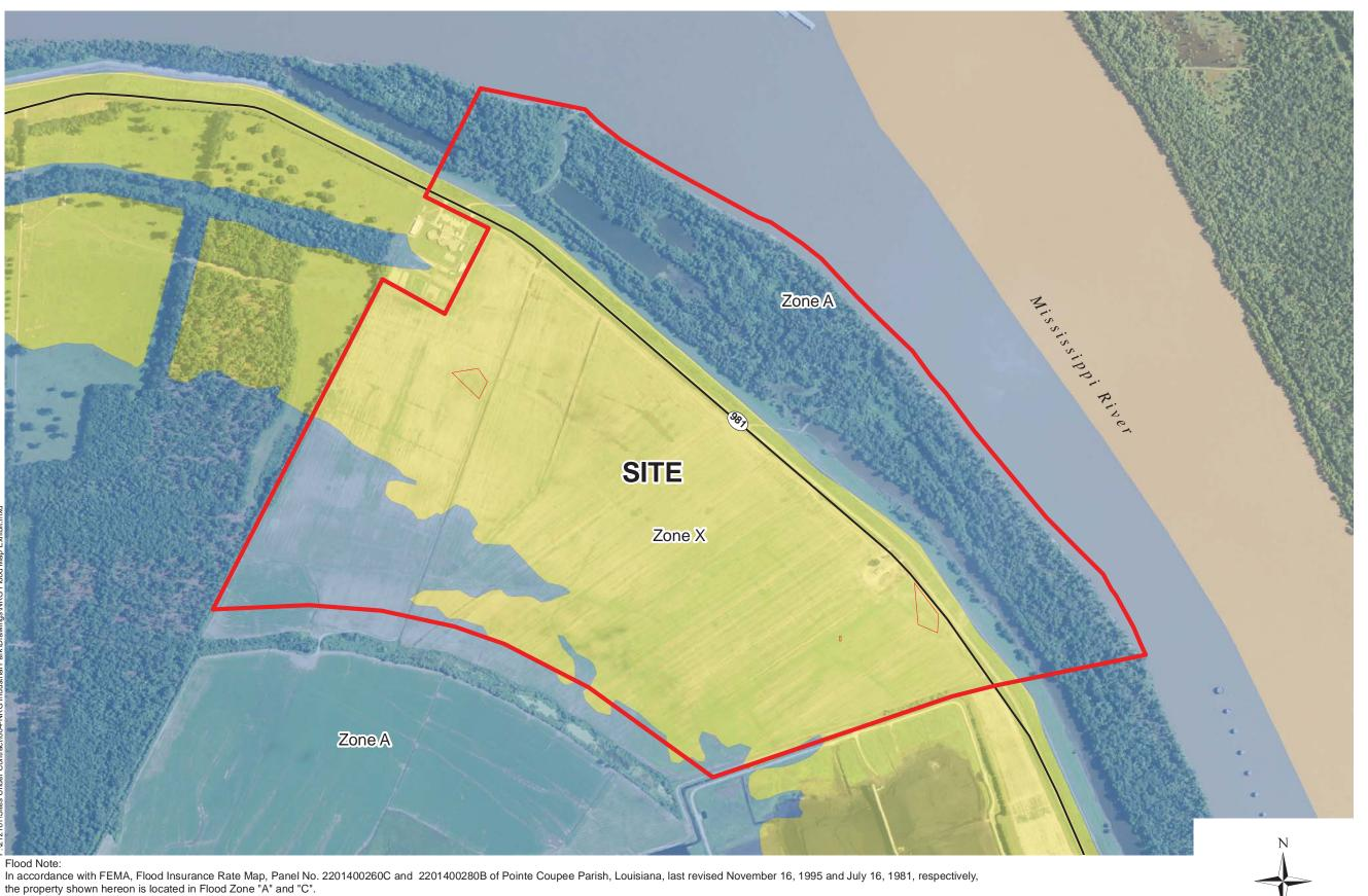
In accordance with FEMA Preliminary DFIRM map, provided by the LSU AgCenter at http://maps.lsuagcenter.com, the property shown hereon is located in Flood Zone "A" and "X". Nearest base flood elevation = 33' (NAVD 1988). Base flood elevation should be verified with the local authority's flood plain administrator
