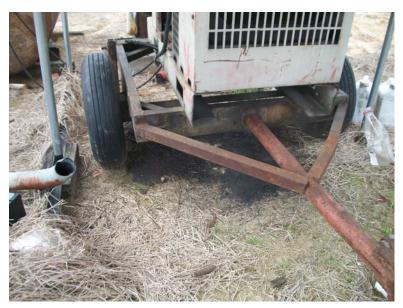
Oil staining below diesel engine.
