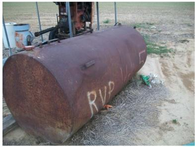
Dent and corrosion on Tank No.2.
