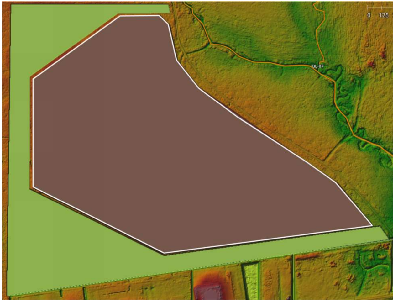
Figure 4 – Potential Layout Alternative 1 (Maximum Allowable Fill Area While Still Meeting Fill Mitigation Requirements)
