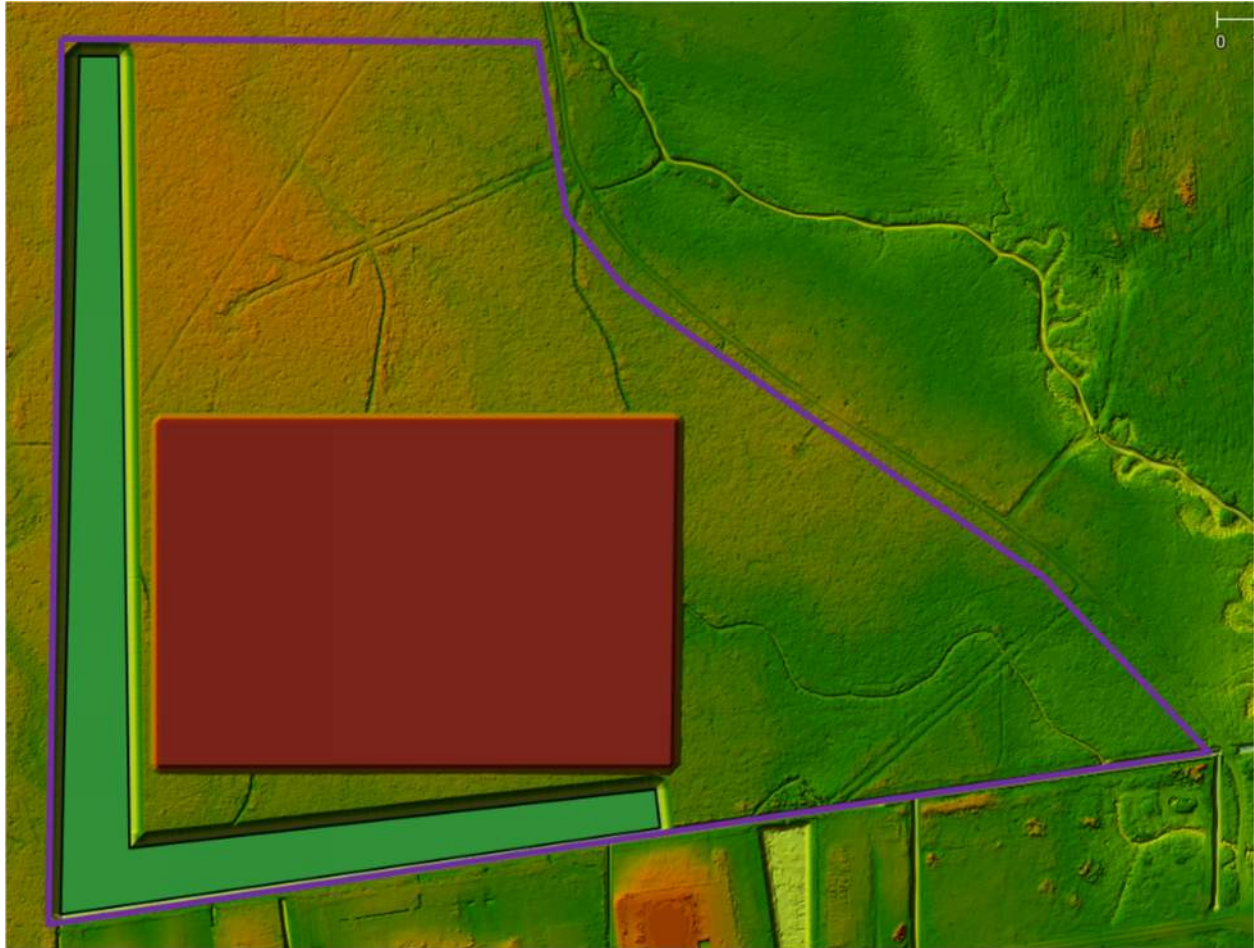
Figure 5 – Potential Layout 2 (1,500,000 sq ft Building and Required Fill Mitigation Pond)
